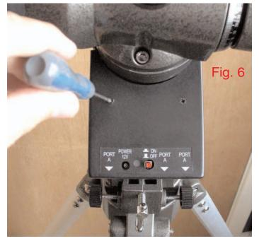
When sliding the plastic cover onto the polar axis drive unit, ensure that the data port connectors slide into their respective holes in the case and that the 12V power connector and red on/off button are visible (Fig. 6). Use two of the small Phillips screws sup-
