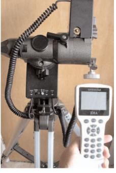
should connect a PORT B on the declination motor to a PORT A on the polar axis motor. Use the other coiled cable to connect another PORT A on the polar axis motor to the white Gotostar hand controller.
