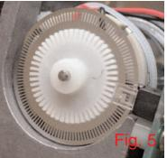
Anything that prevents the encoder from accurately counting the number of shaft revolutions will ultimately affect the pointing and GoTo accuracy of your instrument. (The same applies to the declination axis encoder.)
